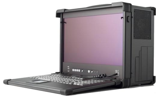
Fig. 1: ACME Portables FlexPAC, the core component in the prototype of the real-time analysis device for microgrids based on instantaneous frequency [1].
